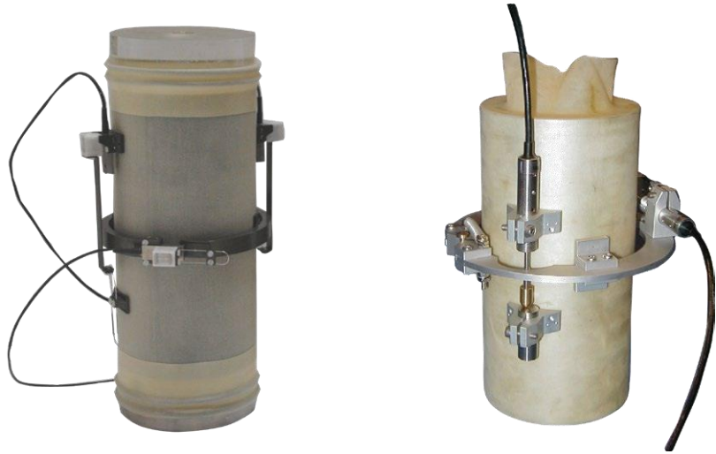
Fig. 11 Hall Effect and LVDT local strain transducers
