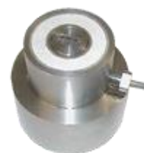
Fig. 2 HAEPD bonded into a bender element triaxial pedestal
