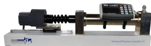
Fig. 5 2MPa/1000cc air pressure/volume controller
