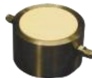
Fig. 1 HAEPD bonded into a standard triaxial pedestal
