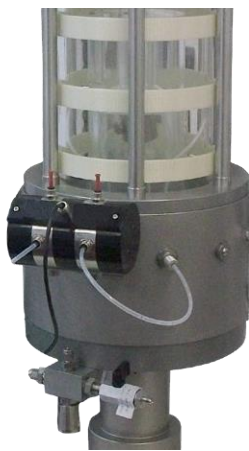
Fig. 7 Ultra low range DPT attached to cell
