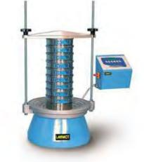
This unit will accept 200, 250, 300, 315, 400 and 450mm, 8 and 12 inch diameter sieves.
