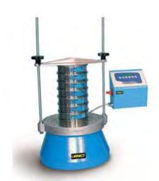
The shaker can hold up to 10 sieves. It is fitted with a digital 1 to 999 minute timer, accessed through the digital control panel. This separate panel also gives the user control of the vibration intensity and pauses between sieving actions, which is particularly useful when sieving fine materials.
