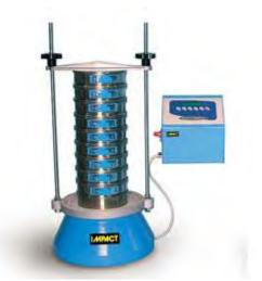
The shaker can hold up to 10 sieves. It is fitted with a digital 1 to 999 minute timer, accessed through the digital control panel. This separate panel also gives the user control of the vibration intensity and pauses between sieving actions, which is particularly useful when sieving fine materials.
