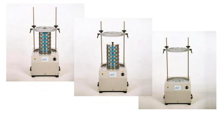
This shaker will accept up to twelve 200mm or 8 inch diameter sieves, lid and receiver or up to six 300mm or 12 inch diameter sieves, lid and receiver.
