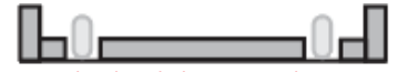
Insulated Track Floor (optional extra TR) Insulation on base floor with inverted tracks for trolleys
